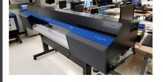
Fab Lab Three Lakes is sporting a few new items this school year, including a Roland TruVis printer/cutter that can be used for vinyl signs, stickers, posters and more. Other new items in the lab include a Ultimaker S5 3D printer; another 3D printer will be added later this fall. Open lab hours are every Tuesday and Thursday from 5 to 9 pm. Stop down and see the new equipment!
